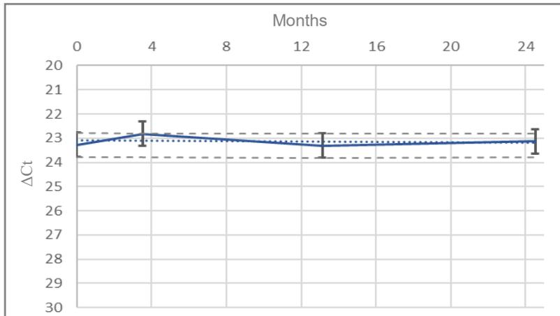
Results illustrate that the Lyo-Ready™ qPCR Mix is active for up to 24 months at room temperature. Lyo-Ready™ Direct DNA qPCR Stool has a projected stable activity up to 12 months. Method error is shown as timepoint standard deviation. Permissible activity interval is shown as dashed lines.
